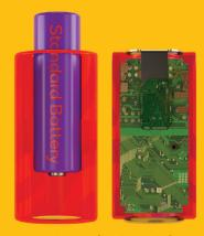
C battery sized. Contains AA battery and IoT hardware.
